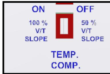
**Figure 4. Setting the Temperature Compensation Switch**
